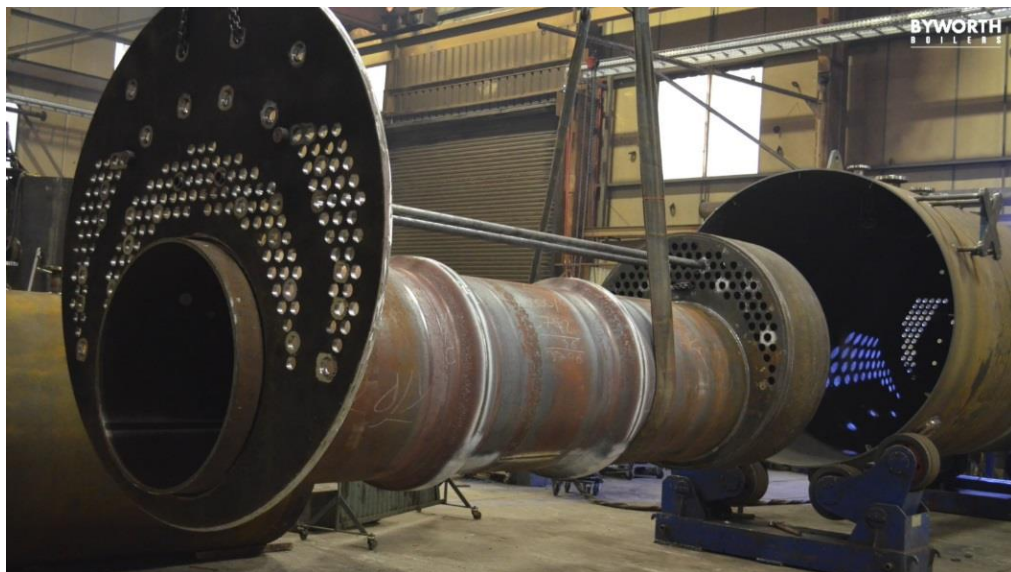
Furnace Tube 800 mm diameter and Tube plate 2.5 metres in diameter being inserted into the boiler shell 5 metres long.
