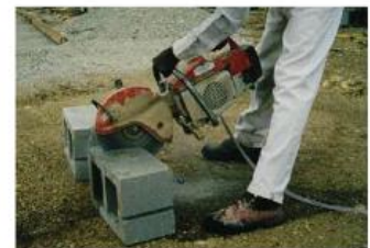
Wet sawing concrete Water is added at saw blade
